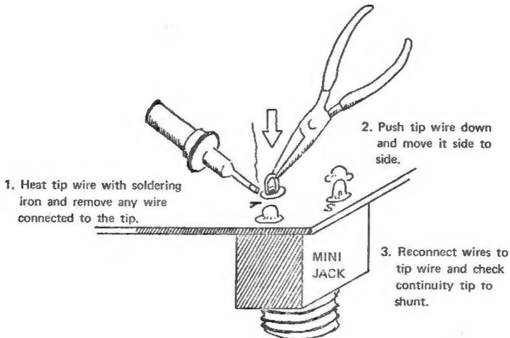
NOTE: See section 6 of the 2600 SERVICE MANUAL for details of mini jack repairs.
