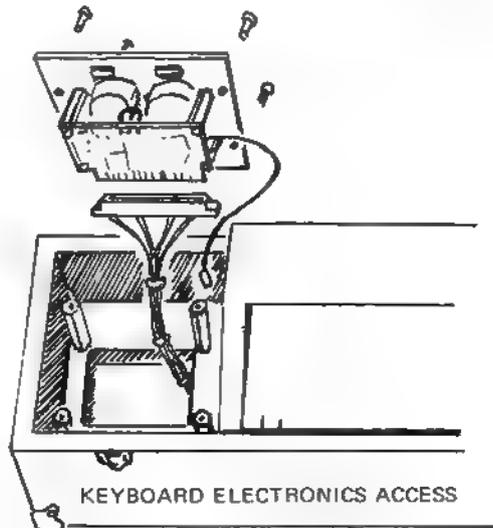
1. If repairs involve only the keyboard electronics, remove the grey metal panel. (see illustration) For proper operation of the keyboard, be sure that this panel does not become grounded since it is at the Keyboard Control Voltage potential.
