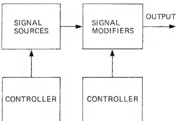
A 'raw' signal is produced by a signal source, such as an oscillator or noise generator. The tone or color of the raw signal is then shaped as the signal passes through the modifier which in the 2600 could be the ring modulator, VCF or VCA. Controllers are used to give automatic variations in the pitch of the signal source and/or the operating characteristics of the modifier.
