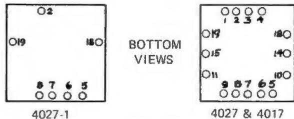
The 4017 and 4027 have from 15 to 18 pins, the 4027-1 has only 7. (Some units containing the 4027-1 may still have the high frequency track trimmer on the board, but it is not connected to the module.)
